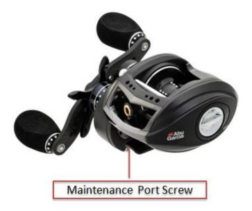
Using a small philips head screwdriver, rotate the screw counterclockwise until free. The small "door" can now be removed. Lightly grease the exposed main gear with quality grease such as <u>Abu Garcia Reel Lube</u>. Once maintenance has been completed, reposition the door over the maintenance port and reinstall the maintenance port screw. Tighten the screw with a philips head screwdriver by rotating it clockwise. Do not over tighten.
